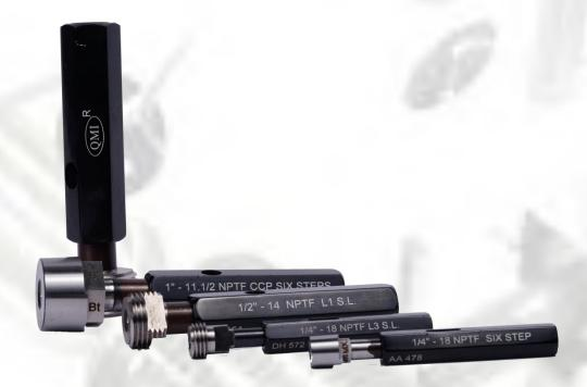
NPTF THREADS can provide pressure tight seal on threads without use of a sealing compound (Dry Seal Type). They are used in pipe assemblies where without using sealing compound pressure tight joint is required on threads. The gauges are intended to be used to test unused pipe threads.
